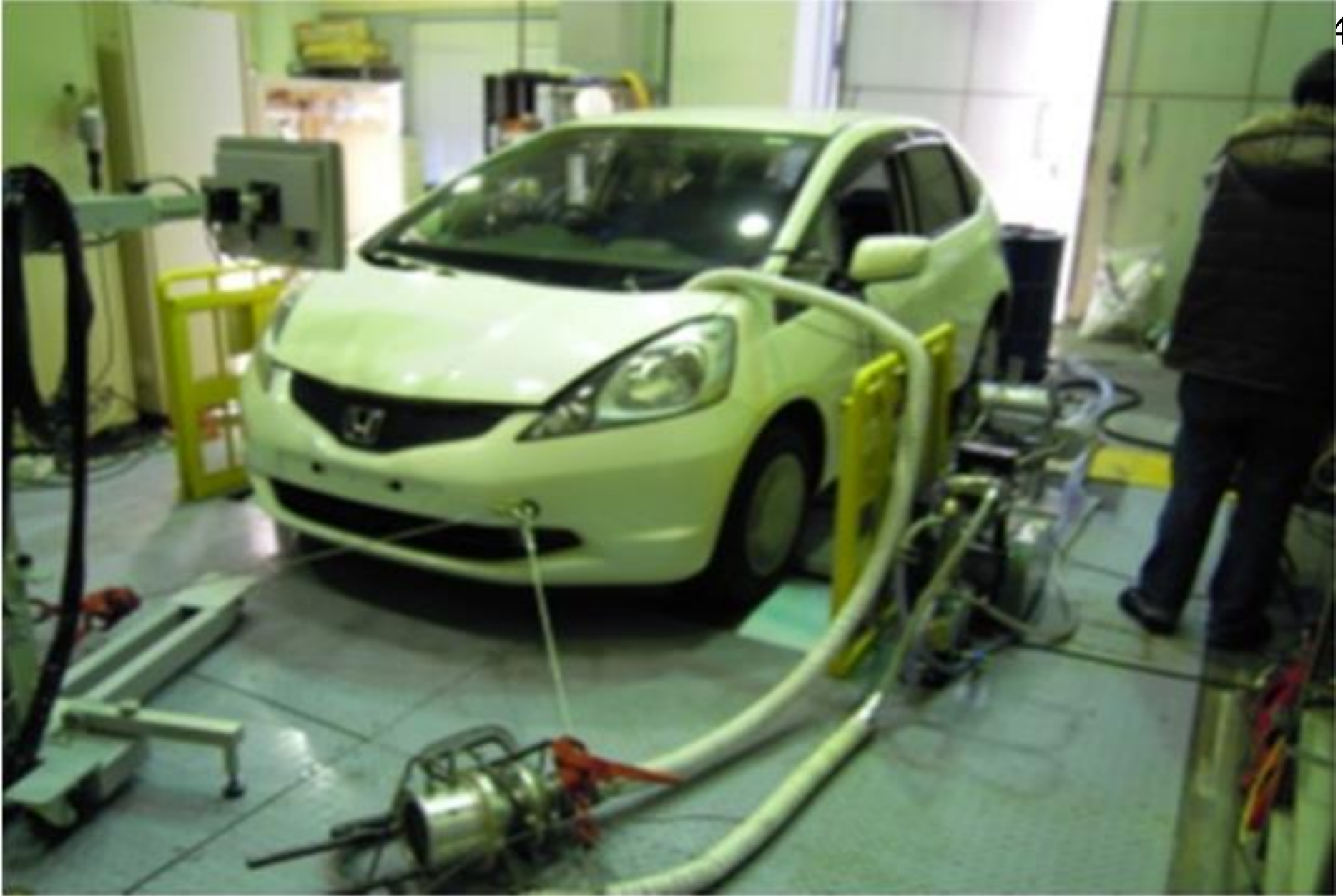
Chassis Dynamometer Evaluation of Catalytic Performance under a Variety of Driving Conditions such as JC08 mode, by Dr. Furutani et al., AIST, Japan
