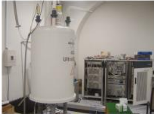
MRI system with superconducting magnet
