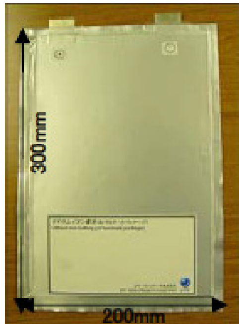
Laminate type cell (capacity: 1.7 Ah)
