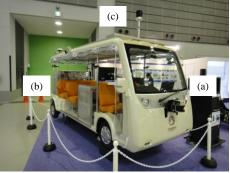
Fig. 2 (a) manufactured large EV, (b) in-wheel motor controller, (c) omnidirectional cameras. Coil for wireless charging is installed under the car.
